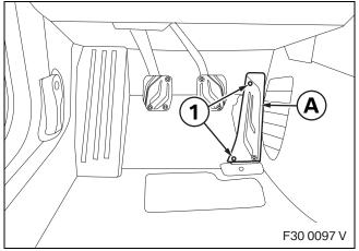
Position M Performance clutch pedal rubber facing **B** on the side and place M Performance clutch pedal stainless steel facing **D** as shown on the clutch pedal (1) and align it appropriately.
