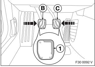
The original facings can be removed from the pedals without the need for any tools. On the clutch pedal (1), slip off the right-hand side and pull the facing to the left. On the brake pedal (2), slip off the left-hand side and pull it to the right. The same essentially applies to the M Performance rubber facings.
