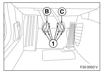
pedal rubber facing **B** and M Performance brake pedal rubber facing **C** using a suitable tool to the pedals.
