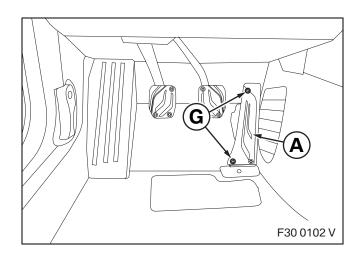
Subsequently press M Performance accelerator pedal stainless steel facing **A** firmly onto the accelerator and screw into position using Torx screws **G**.
