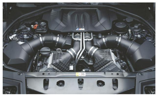
There is a new air duct both for the center radiator package and for the side M-specific low-temperature radiator. The lower engine compartment shielding is one-piece for stiffness reasons (instead of 3-piece). It includes the exhaust air duct of the engine oil cooler and improves aerodynamics. The lower bumper support is plastic (saves on weight) and is secured to the M6-specific deformation elements. The shaped element in the upper bumper support is adapted to the shape of the M6 bumper panel.
