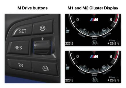
While driving in one of the M configuration modes and the ignition is switched off the M button must be reselected when the ignition is switched back on in order to reactivate the M mode. The M1 or M2 symbol in the instrument panel goes out when deactivated
