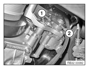
Release screws (1) and remove power steering pump (2) and turn far enough to the side to be able to release screw connection of pressure line.
