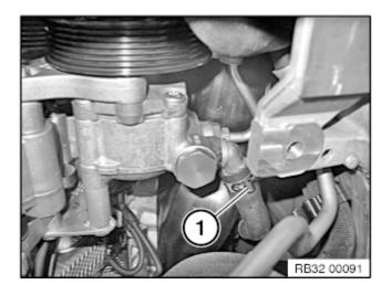
Release hose clamp (1) and detach suction line from power steering pump. *Installation note:* Replace hose clamp.
