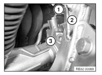
Release screw (1) and lines (3) and (2) pull off. *Installation note:*Replace sealing rings.
