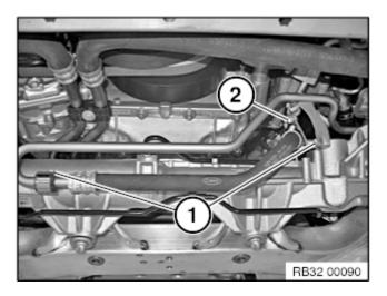
Release screws (1) and nuts (2) of holder on steering gear.
