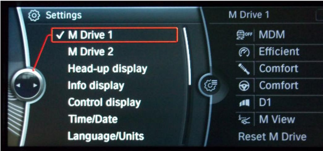
The settings can be selected by pressing the corresponding button on the multifunction steering wheel. The two M buttons on the steering wheel allow the driver to select between two different M Drive modes that can be saved and activated.
