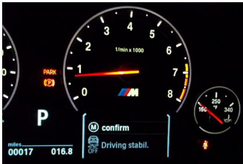
If the DSC selection of "MDM" or "DSC OFF" is selected, a second actuation of the corresponding M button is required to activate the M configuration as a confirmation for M mode for safety reasons.
