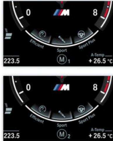
While driving in one of the M configuration modes and the ignition is switched off the M button must be reselected when the ignition is switched back on in order to reactivate the M mode. The M1 or M2 symbol in the instrument panel goes out when deactivated
