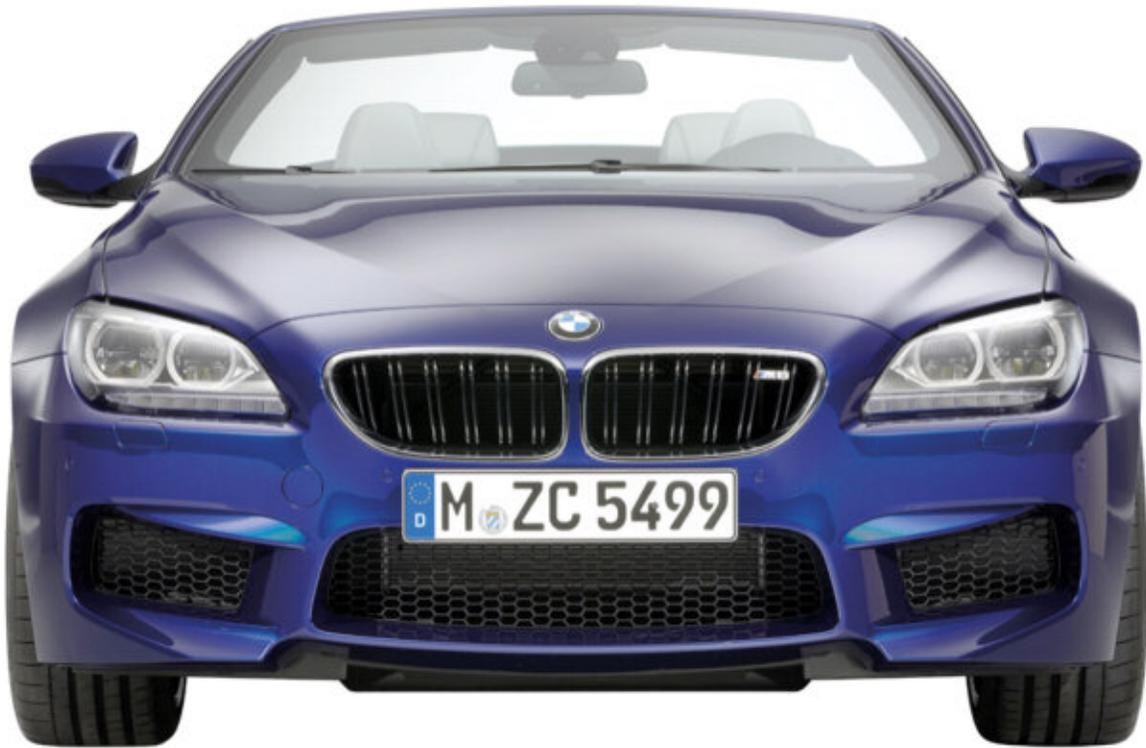
The bumper has been designed specifically for the M6. The lower area of the bumper reduces lift at the front axle. The PDC sensors are painted in the vehicle color. No fog lights are installed due to the large air inlets.
