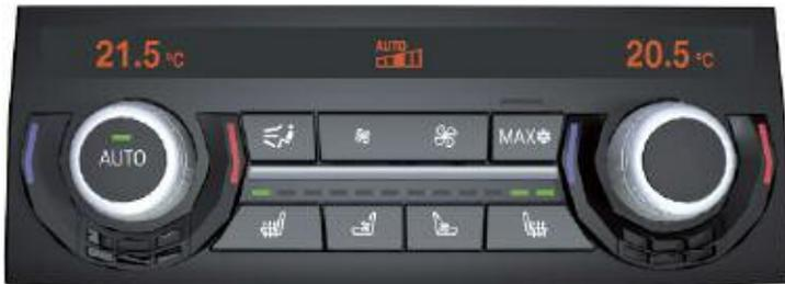
The rear passengers can adjust the temperature separately for the left and right sides of the rear passenger compartment.
