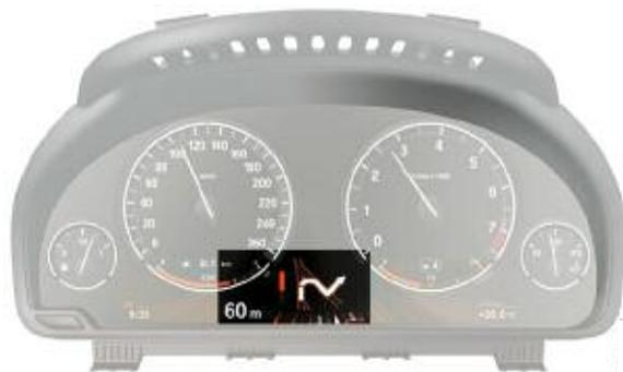
**Navigation-system display in the instrument panel**
