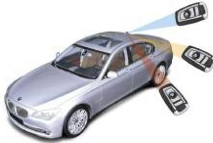
The individual settings in the vehicle are stored automatically when the user leaves the vehicle. As soon as the vehicle is unlocked using the identification transmitter, the system recognizes the corresponding settings belonging to that transmitter. Up to three different basic settings can be adapted for three different identification transmitter.
