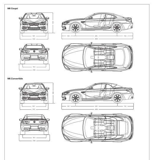
All dimensions of technical drawings in millimetres. Luggage compartment volumes: Coupé 460 litres, Convertible 300 to 350 litres (with folded up roof storage box).
