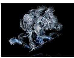
M TwinScroll turbocharger with a cross-bank exhaust manifold: the exhaust flows from each of two cylinder pairs with a 360° firing interval are combined and routed along separate channels before reaching the turbine wheels of the turbochargers. This guarantees that gas flow is not compromised. It's a highly efficient charging concept that leads to optimum energy transfer - and, therefore, extremely spontaneous responsiveness.
