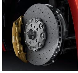
M carbon ceramic brake system:1 the high-performance lightweight brakes in the BMW M6 Coupé and Convertible have extremely high load capacity and excellent resistance to fade. The system can be identified by the matt gold-painted brake calipers with M logo.
