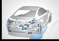
Active M Differential: this optimises traction at full power even in tight bends, during high-speed cornering and on variable road surfaces. An electronic control unit links the active system and DSC and proactively ensures the intelligent use of locking torque in every driving situation. In this way, no drive power is wasted and perfect handling is guaranteed.
