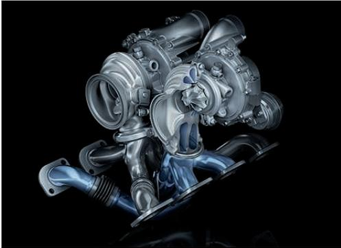
**M TwinScroll turbocharger with a cross-bank exhaust manifold:** the exhaust flows from each of two cylinder pairs with a 360° firing interval are combined and routed along separate channels before reaching the turbine wheels of the turbochargers. This guarantees that gas flow is not compromised. It's a highly efficient charging concept that leads to optimum energy transfer – and, therefore, extremely spontaneous responsiveness.
