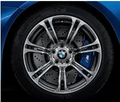
■ **19" M light-alloy wheels Star-spoke 344 M**, forged and polished, with mixed tyres. Front: 9.5 J x 19 with 265/40 R 19 tyres. Rear: 10.5 J x 19 with 295/35 R19 tyres.
