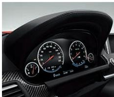
■ **Extended instrument cluster** with Black Panel display with permanently illuminated white surrounds for speedometer and rev counter plus fuel level and oil temperature displays.
