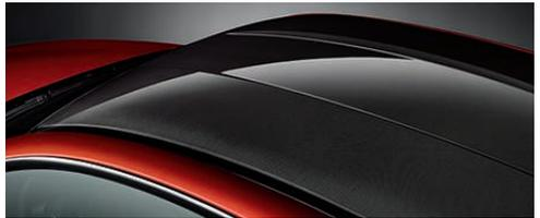
■ **The carbon roof** of the new BMW M6 Coupé is in carbon fibre reinforced plastic. It is very light and extremely stiff.
