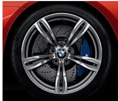
□ **20" M light-alloy wheels Double-spoke 343 M**, forged, with mixed tyres. Front: 9.5 J x 20 with 265/35 R 20 tyres. Rear: 10.5 J x 20 with 295/30 R20 tyres.
