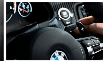
The seven-speed M Double Clutch transmission with Drivelogic can be shifted using the paddles, and you don't need to take your foot off the accelerator, for an even sportier driving experience.
