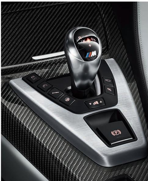
■ **Gear lever** for seven-speed M Double Clutch Drivelogic transmission, with M logo and illumination.
